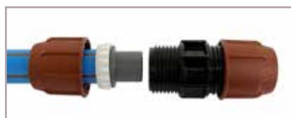
Push the barbed end of the adaptor into the pipe until it meets the stop (a mallet may be required). Then push the plain end of the adaptor into the fitting until it meets the stop.
